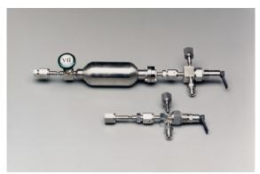
The unique features of these proprietary PSO Calibrated Leaks result in their use in a wide variety of applications. They are extensively used for verification tests and calibration of Leak Testing Systems, usually with automated valve operation and usually with an external gas source rather than a reservoir. They are also used frequently to flow gas at a controlled
